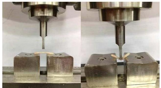
**Figure 3:** *The test specimen is deflected in this way at a constant rate until rupture occurs at the other surface of the specimen.*
